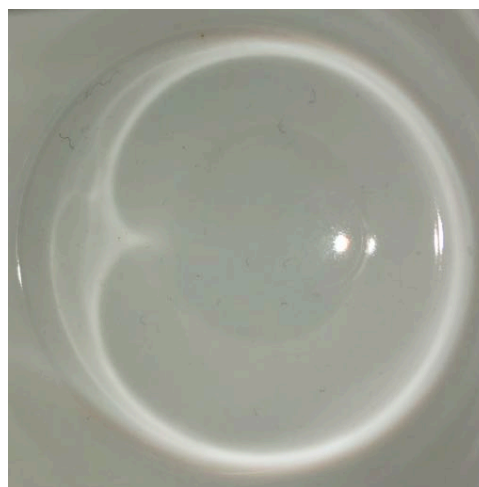
Figure 2. Shine a light from the edge of a coffee cup and the caustic it forms is a cardioid.
